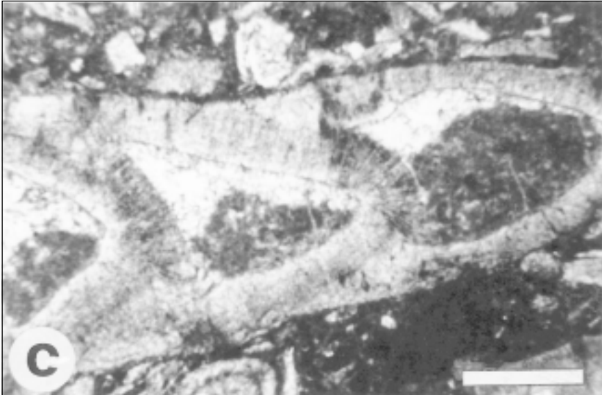
PLATE 3C. Discocyclinal nummulitic packstone with close up view of longitudinal axial section of Assilina sp. showing geopetal infillings. Scale bar = 250 \mu m.
